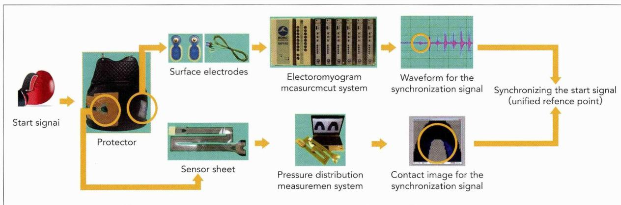
Fig. 6 System for synchronization between electromyogram measurement system and pressure distribution measurement system.
