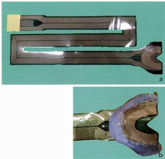
Fig. 4 Custom sensor sheet. (a) Custom sensor sheet for measuring occlusal contact. (b) Silicone impression for holding custom sensor sheet.
