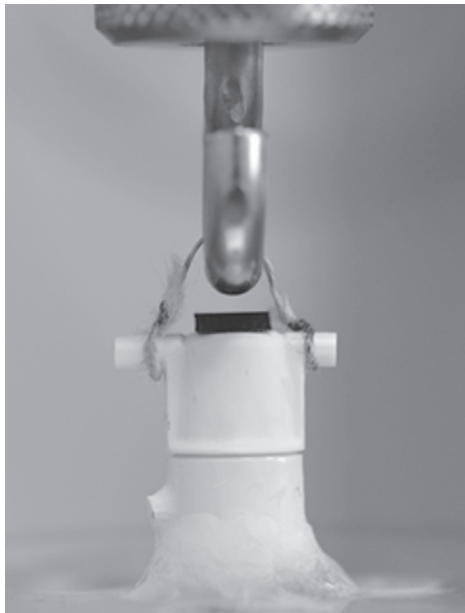
Fig. 2 Measurement of retentive force.
