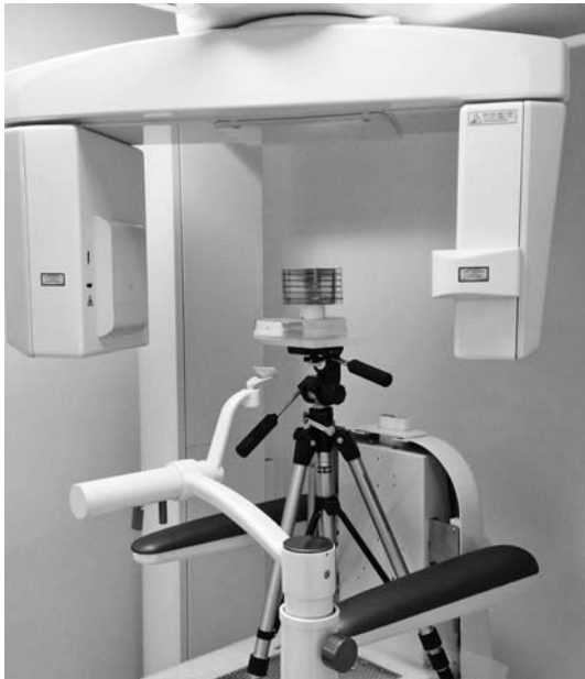
Fig. 4 Phantom mounted on the 3D Accuitomo F17.
