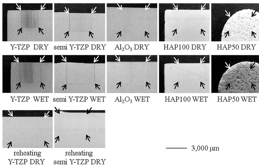
Figure 5 Observation photograph of the laser irradiation trace of the sample surface
