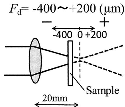
Figure 2 Position relations schematic view of defocused distance:  $F_d$
