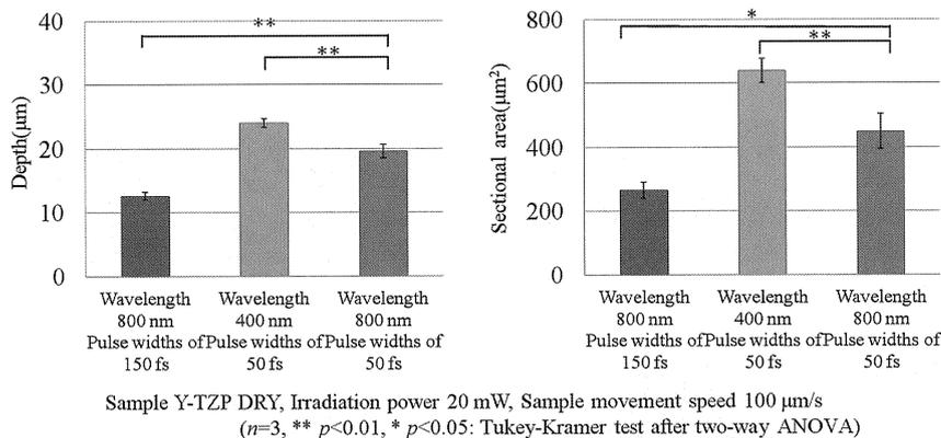
Figure 8 Dependence of the maximum trace depth and sectional area on the wavelength and pulse width
