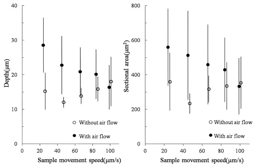
Sample Y-TZP DRY, Wave length 400 nm, Pulse widths 50 fs,  $F_d$  -200 μm, Irradiation power 20 mW ( $n=3$ )
