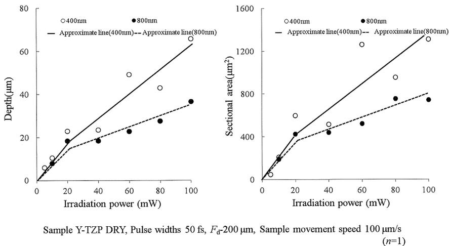
Figure 7 Dependence of the trace depth and sectional area on the irradiation power
