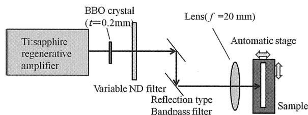
Figure 1 Experimental setup for processing ceramic samples
