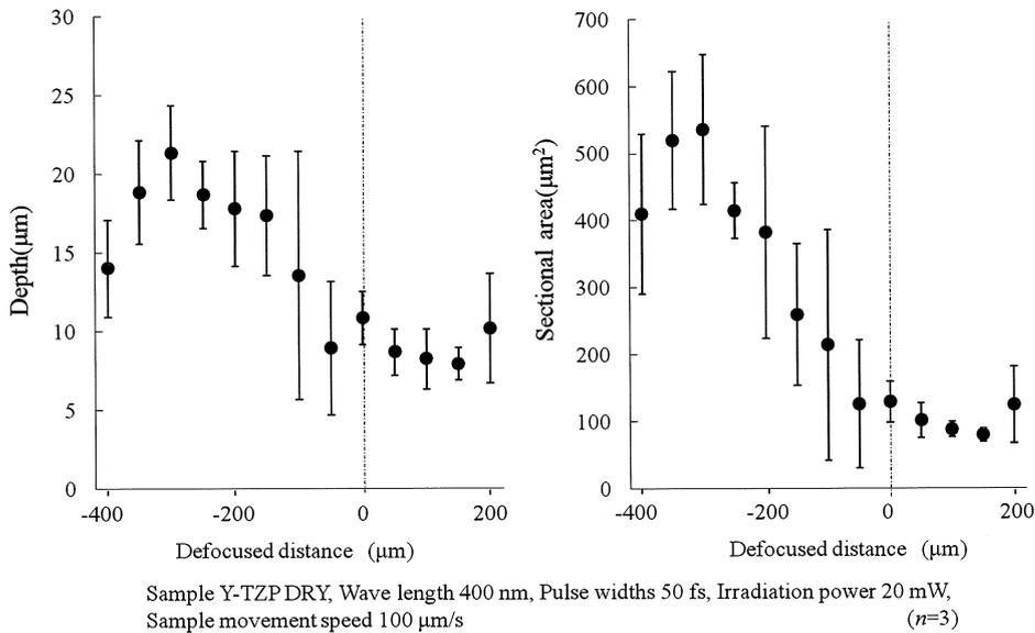
Figure 3 The relationship between the defocus distance and the depth and sectional area of the irradiation traces
