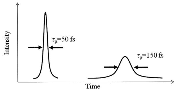
Figure 10 Comparison of peak intensities of laser pulses with the same pulse energy, however with different pulse widths of 50 and 150fs
