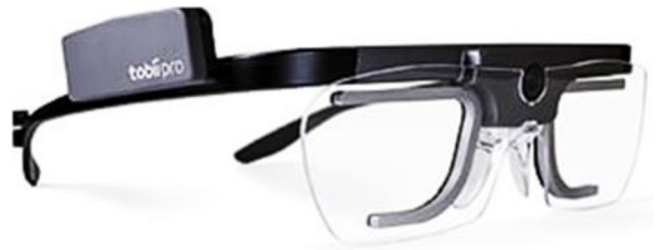
Fig. 1. Measuring equipment. Tobii pro/glasses 2 (Tobii Technology Japan, Ltd., Tokyo, Japan) was used.
