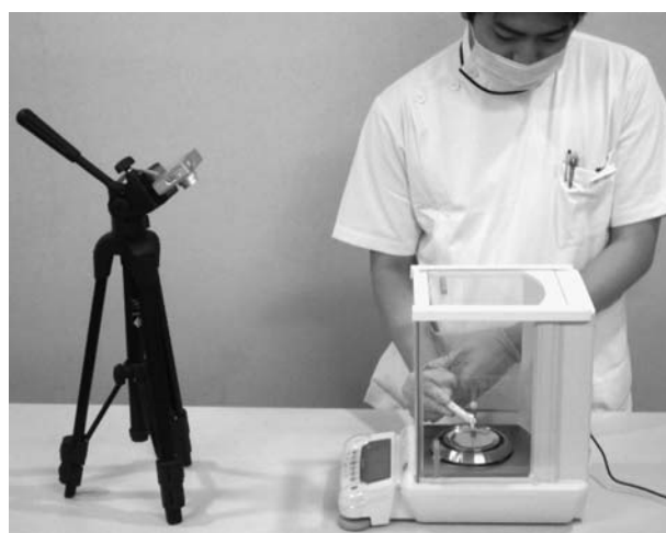
Fig. 2 Measurement of the load value with a modified SW monofilament.
