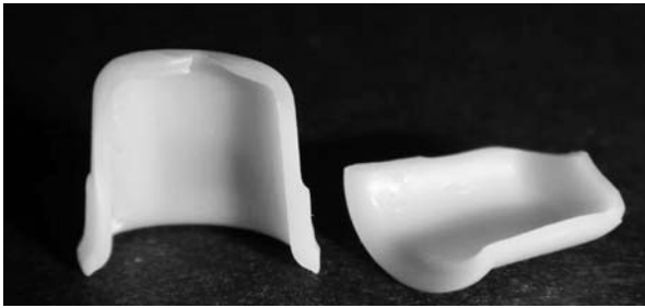
Fig. 6 Representative fracture mode of secondary crowns.
