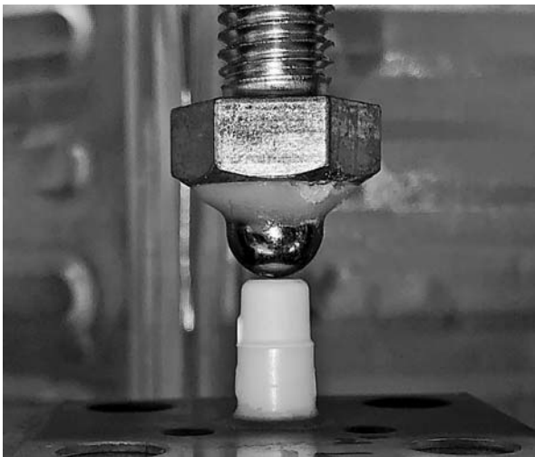
Fig. 4 Measurement of fracture strength.
